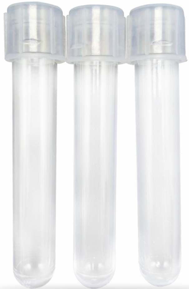
12 X 75 MM TUBES OF 5 ML CAPACITY
